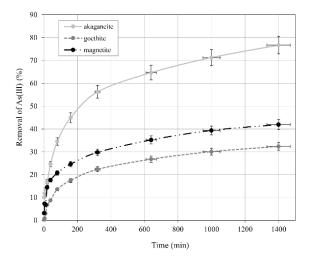
Fig. 4. Adsorption of As(III) onto iron-based adsorbents as a function time (100 mg dm<sup>-3</sup>; 25 °C; dose of adsorbent 25 mg; pH 4.5)
