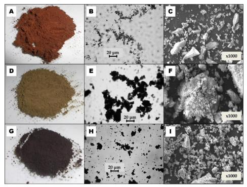
Fig. 1. Images of synthetic iron-based minerals taken with a digital camera (A, D, G), an optical microscope (B, E, H) and a scanning electron microscope (C, F, I); viewed from above: akaganeite (A-C), goethite (D-F) and magnetite (G-I)
