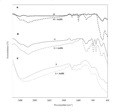
Fig. 7. FTIR spectra of synthetic iron-based minerals before and after As(III) adsorption: A – magnetite; B – goethite; C – akageneite
