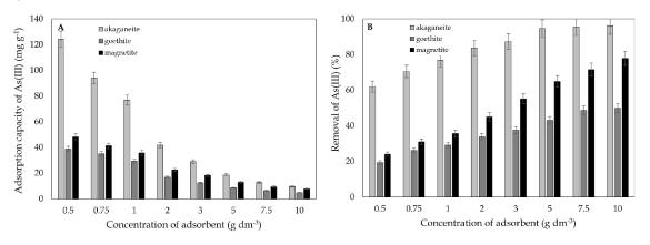
Fig. 2. Effect of adsorbent dose at 100 mg dm<sup>-3</sup> of initial As(III) concentration on: A – adsorption capacity of As(III) and B – removal of As(III)
