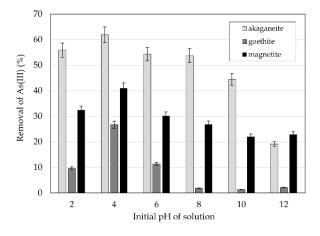
Fig. 3. Adsorption of As(III) onto iron-based adsorbents as a function pH (100 mg dm<sup>-3</sup>; 25 °C; dose of adsorbent 25 mg)
