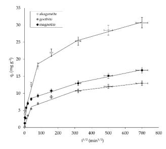
Fig. 5. Intraparticle diffusion model of As(III) adsorption on iron-based minerals (100 mg dm<sup>-3</sup>; 25 °C; dose of adsorbent 25 mg; pH 4.5)
